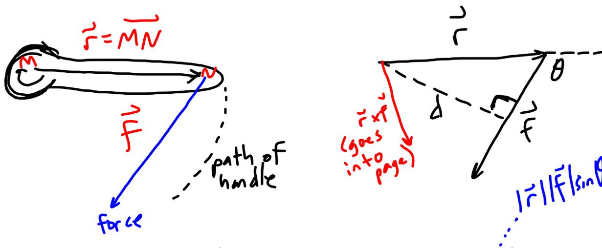
The torque, or the turning effect, of the force  $\vec{f}$  about the point M is defined to be the vector  $\vec{r} \times \vec{f}$ . This vector is perpendicular to the vectors  $\vec{r}$  and  $\vec{f}$ . To find its direction, we used a right-hand grip rule as follows: If you grip the imaginary axis of rotation at the point M so that your fingers point in the direction of the force, then your extended thumb points in the direction of the torque vector.
